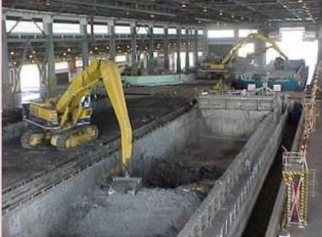
Large excavators with specially designed, interchangeable grabs unload the solid waste from the barge directly into 35-tonne payload off-road dump trucks.
