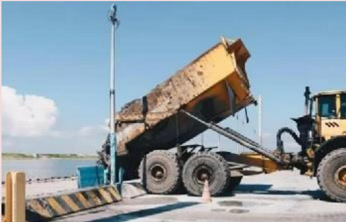
The dump trucks make their way to the designated tipping site and unload the solid waste into an active cell. Bulldozers and compactors then level and compact the solid waste.
